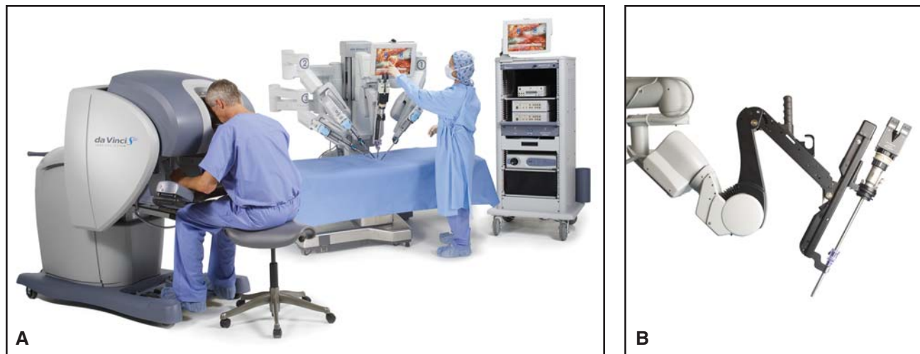
Fig 3A-B. — The da Vinci Surgical System. (A) The surgeon is seated at the console at a short distance from the patient-side cart with the four interactive robotic arms and the vision system. (B) A robotic arm uses instruments that provide seven degrees of freedom. Photos courtesy of Intuitive Surgical, Inc, 2008.
